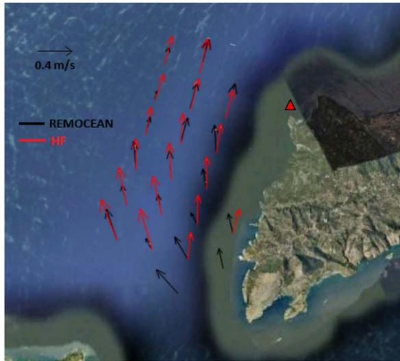
Fig. 5. Map of the sea surface currents estimated by REMOCEAN system and measured by the HF radar on February 17, 2010. The red triangle indicates the position of the HF-radar antenna.
