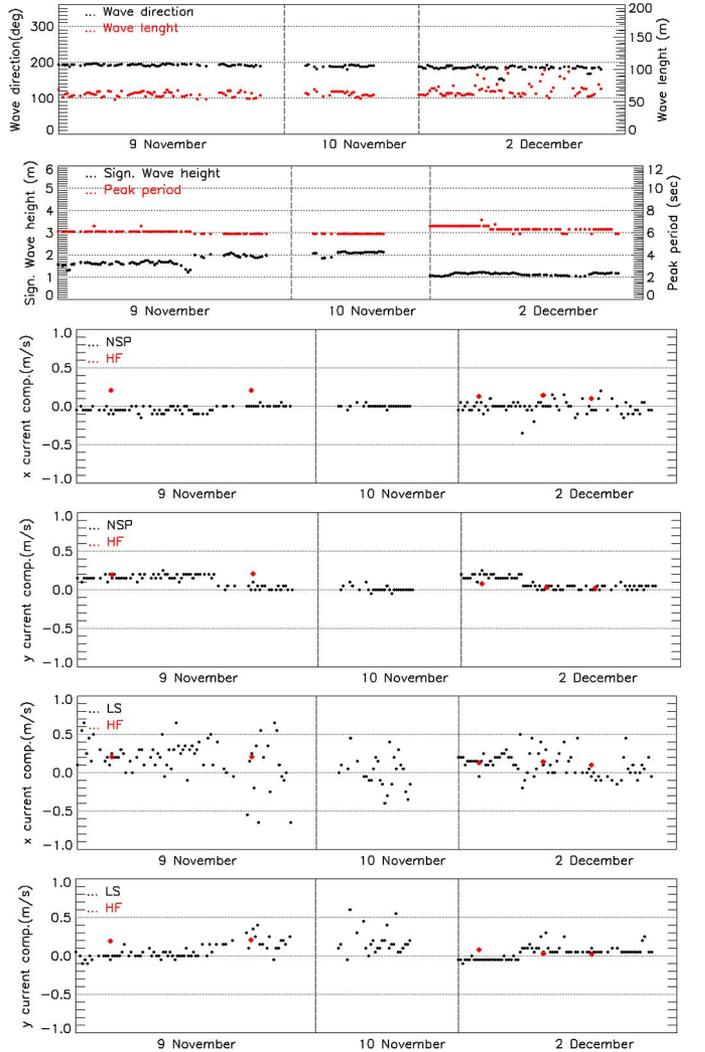
Fig. 3. Sea-state parameter estimates provided by the REMOCEAN system for the first site in Naples. The red diamonds represent the HF-radar measurements.
