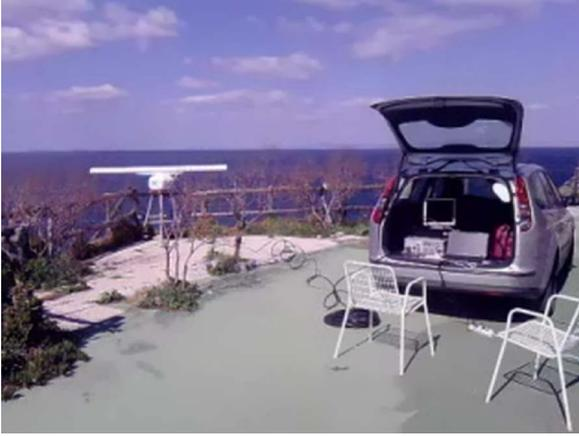
Fig. 1. REMOCEAN system in mobile modality acquisition on the Gulf of Naples coast.
